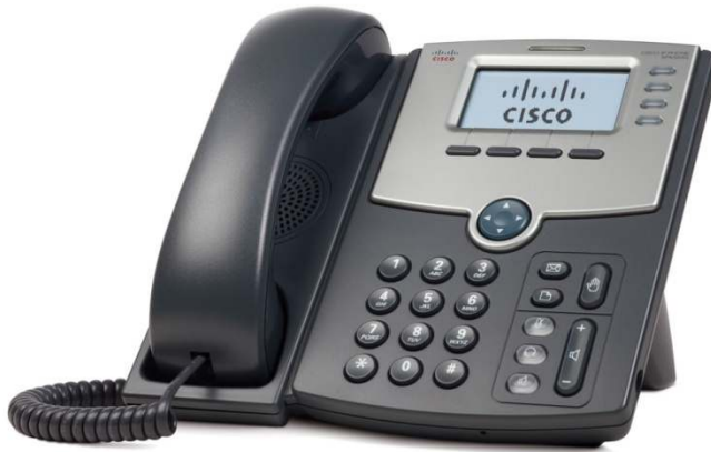
Figure 1. Cisco SPA504G 4-Line IP Phone
